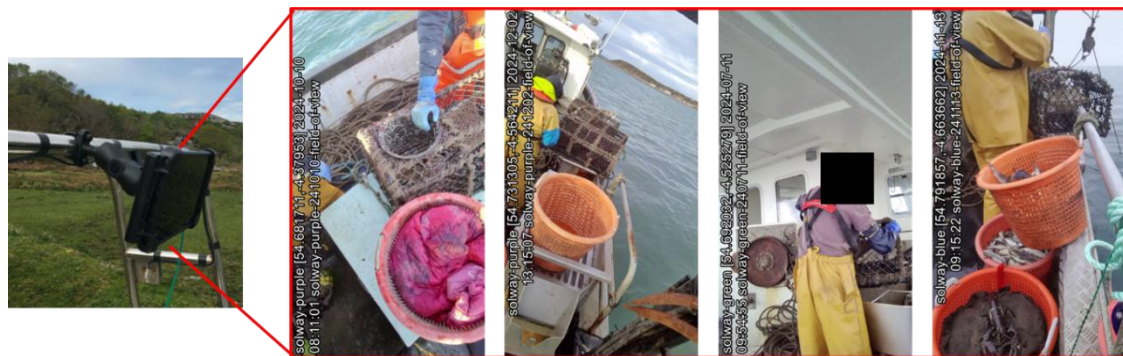
Figure 2 . The EM tablet system mounted on a boat railing, and examples of the field of view from the tablet.
